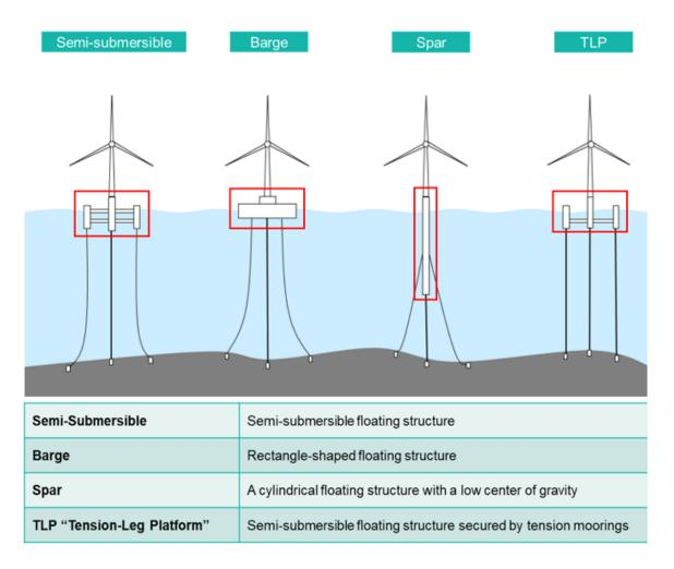
Major floating structure technologies for offshore wind turbine (enclosed sections)
