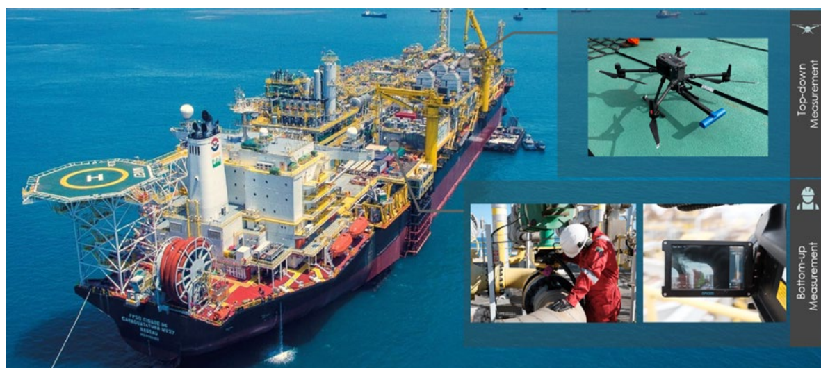
Figure 1: Measuring methane at an FPSO
