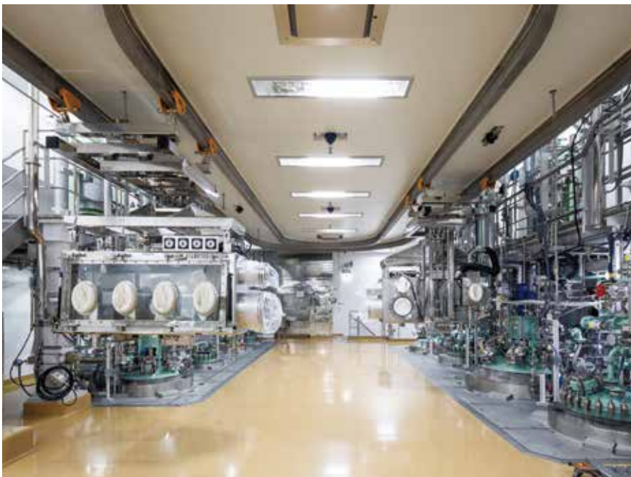
A facility with an advanced containment technology in the mid-sized API manufacturing facility of Chugai Pharmaceutical Co., Ltd. This technology ensures worker safety from exposure to highly potency compounds.
