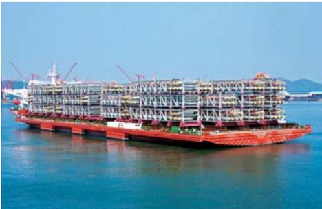
Pre-assembled modules aboard a module carrier,
