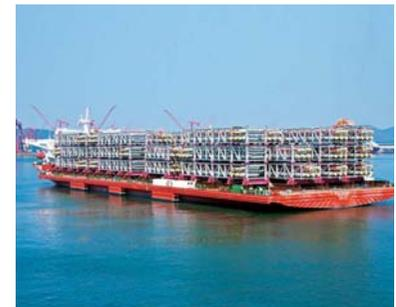
Pre-assembled modules aboard a module carrier, image courtesy of the Chevron-operated Gorgon Project
