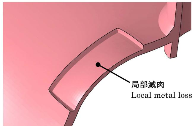
Fig. 6 Analysis Model of Local Metal Loss around Equipment Nozzle
