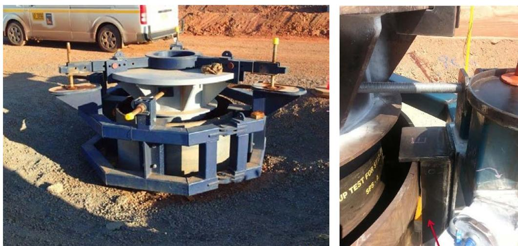
Fig.8 Setting Jig for Steel Socket
