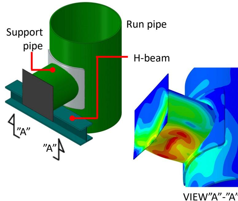
Deformation of support by elastic-plastic analysis
