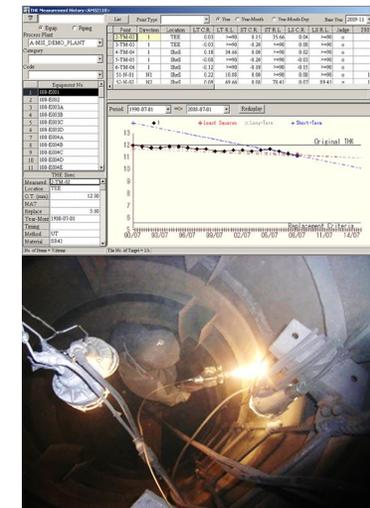
Inspection Result and Thermal Spray Coating for Life Extension
