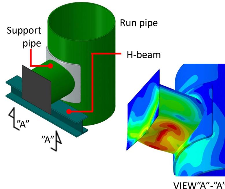
Deformation of support by elastic-plastic analysis
