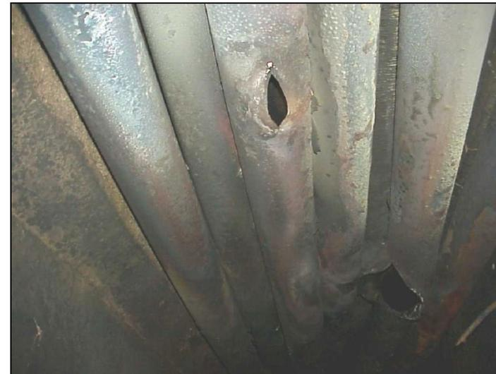
Creep rupture of furnace tube
