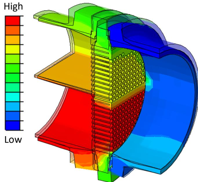
Temperature distribution and deformation of flange
