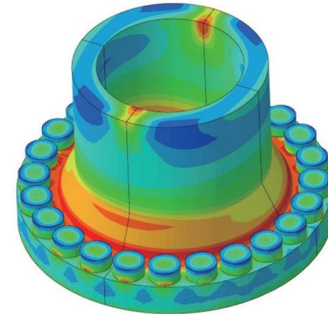
(2) Stress Distribution in Flange Caused by Bolt Tightening
