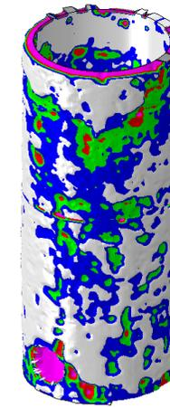
(1) External Corrosion Analysis Model by Laser Scanning
