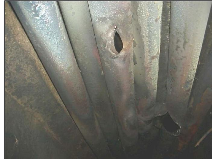
Creep rupture of furnace tube
