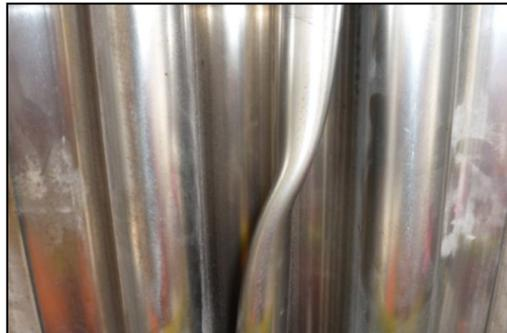
Deformed expansion joint
