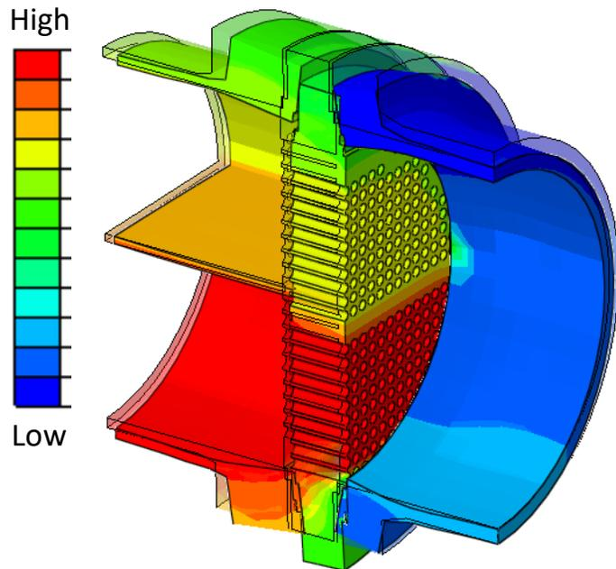
Temperature distribution and deformation of flange
