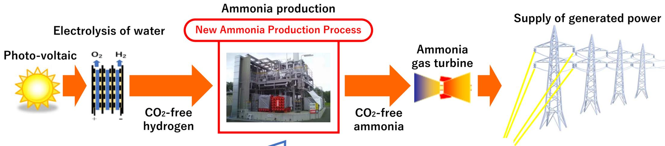
Production of CO<sub>2</sub>-free ammonia with the demonstration test plant using the new ammonia synthetic catalyst developed in May this year.
