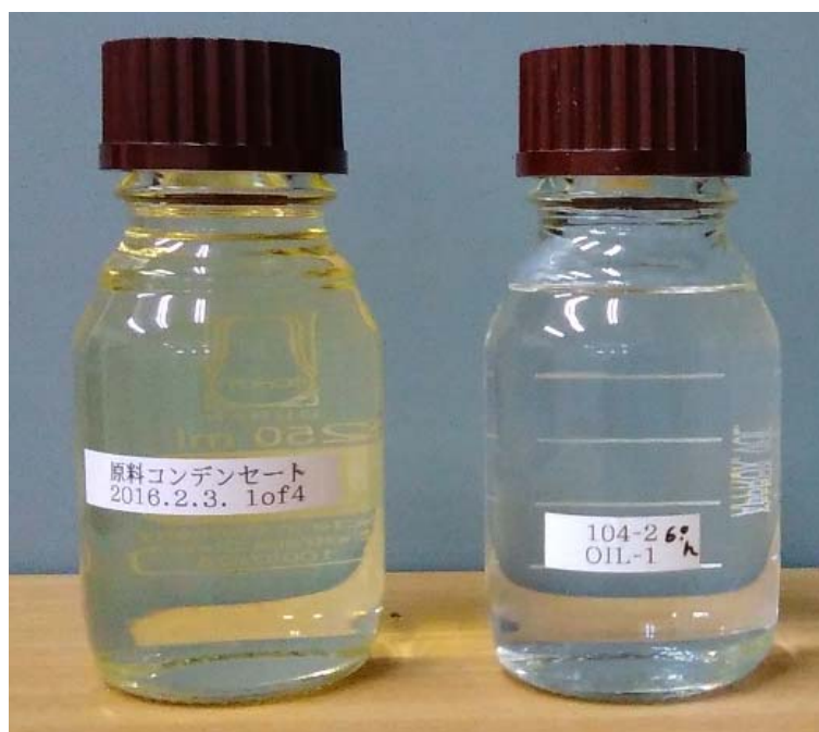
Fig. 6 Comparison of Feed and Product Condensate, Left: Feed Condensate (before reaction), Right: Product Condensate (after reaction)
