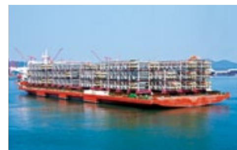
Pre-assembled modules aboard a module carrier, image courtesy of the Chevron-operated Gorgon Project
