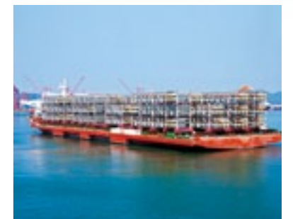
Pre-assembled modules aboard a module carrier, image courtesy of the Chevron-operated Gorgon Project
